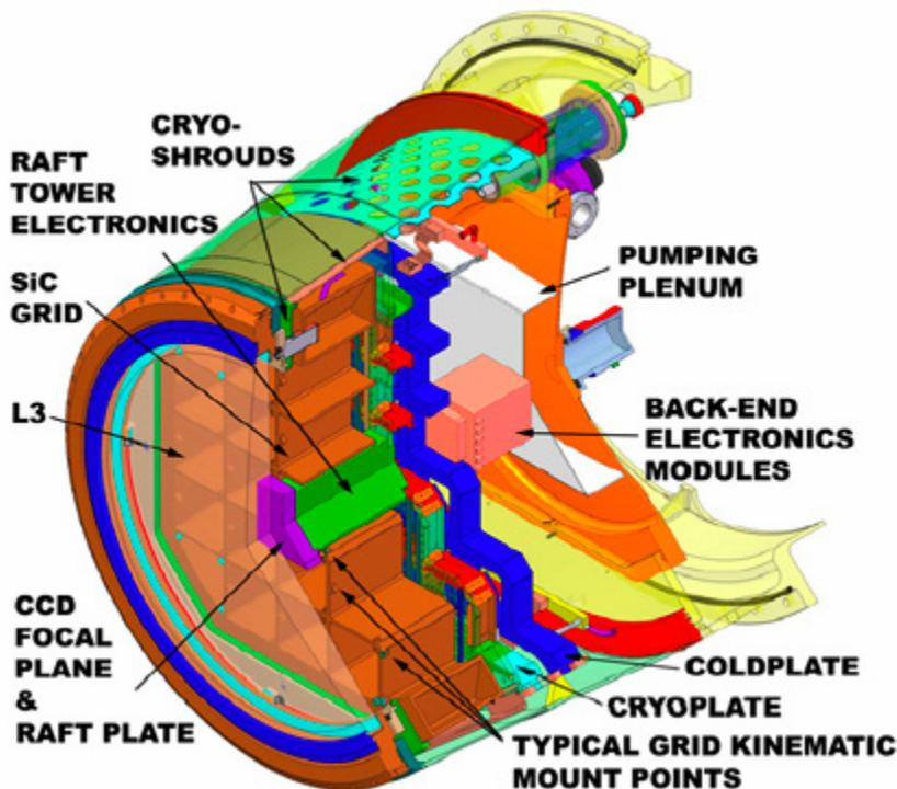
**Figure 1.** Cross section of the cryostat. SiC: Silicon carbide. L3: Third lens in the optical train.
